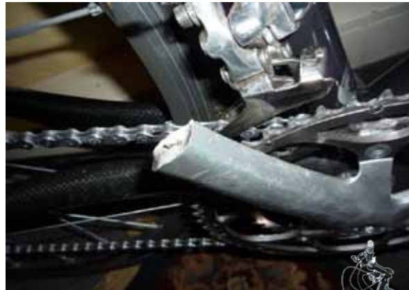
Bicycle crank shaft broken due to fatigue
