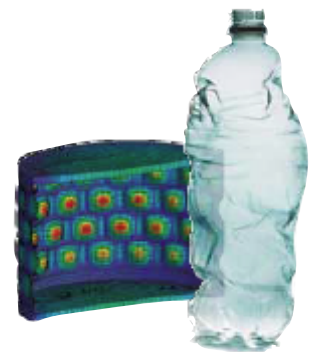
Nonlinear stability analysis of stiffened structure subjected to internal pressure
